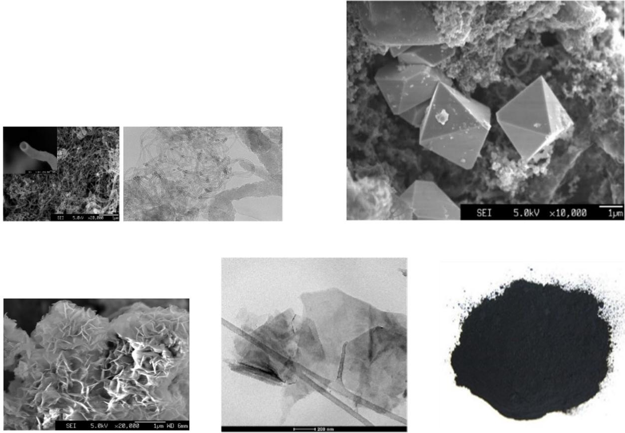
Figure 3: A. TEM and SEM images of MWCNTs obtained experimentally by electrolyses in molten salts at the Faculty of Technology and Metallurgy in Skopje; B. TEM and SEM images of graphene obtained experimentally by electrolyses in molten salts at the Faculty of Technology and Metallurgy in Skopje; C. Nanodiamonds obtained by electrolyses in molten salts; D. Graphene and CNTs in natural dimensions.
