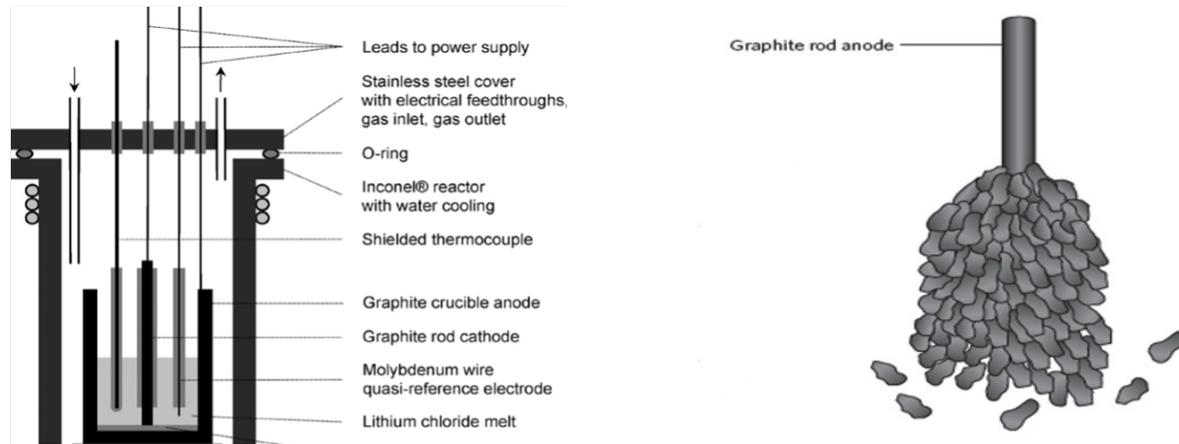
Figure 2: Direct exfoliation of graphene. Schematic of experimental set-up used for conventional electrolysis
